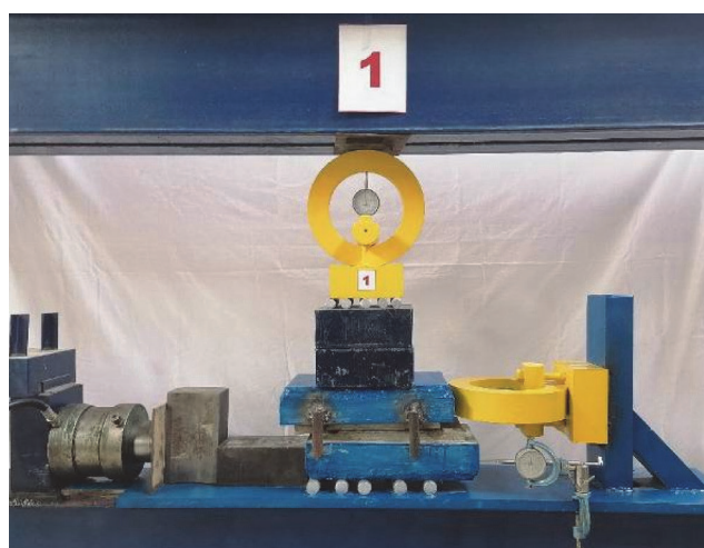
Figure 8. View of the apparatus during the experiment (visible shearing of upper and lower half of the specimen)
