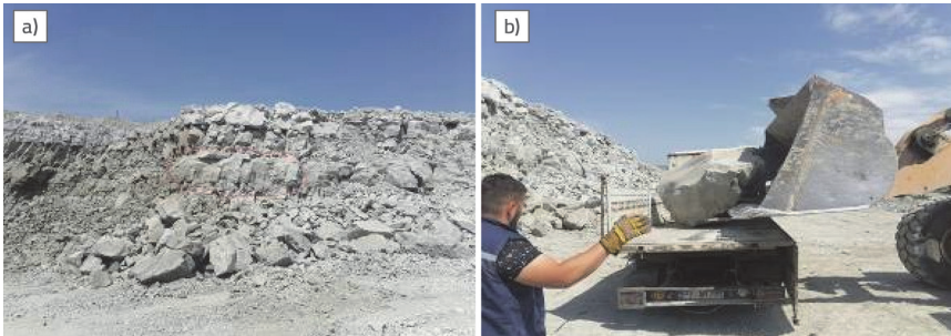
Figure 1. a) position of a bench from which the rock mass block was extracted, b) loading of the rock mass block
