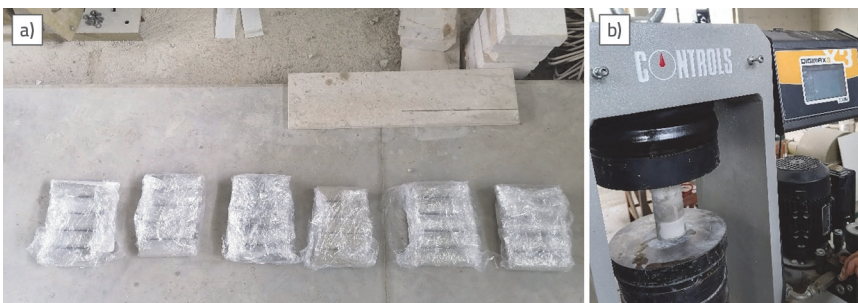
Figure 3. Examination of uniaxial strength of specimens
