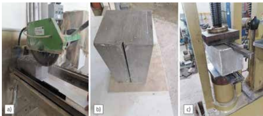
Figure 4. a) Cutting a groove at the specimen centre; b) Cut groove of 1 cm depth; c) Forming of discontinuity
