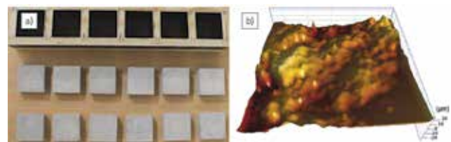
Figure 6. Details of concrete blocks: a) concrete samples and plywood molds b) surface roughness measurement sample
