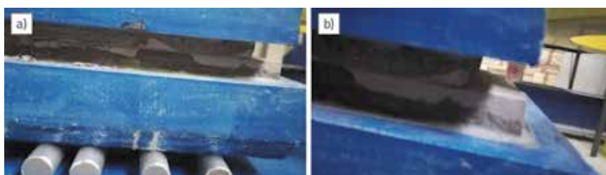
Figure 9. Displacement of upper half (a) in relation to the lower half (b) of the specimen along the shear surface
