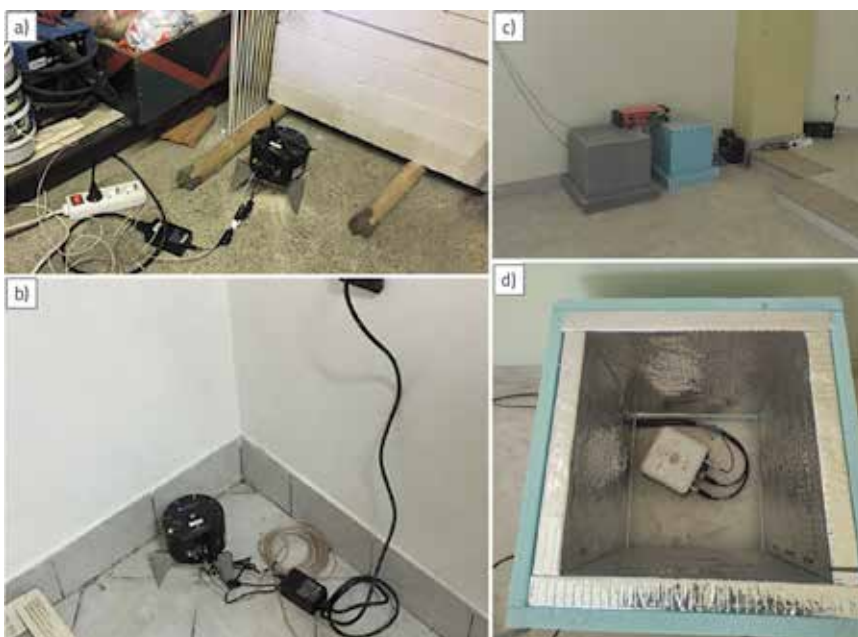
Figure 3. Examples of installed temporary stations: a) Temporary stations in Sisak; b) and Taborište equipped with a short period instrument (seismograph with integrated accelerometer Lunitek Sentinel-Geo ) from rapid deployment of the OP-Net; c) Temporary station in Petrinja cemetery of the Petrinja-Net with collocated seismometer Kinemetrics MBB-2 (grey insulation box) and accelerometer Kinemetrics ETNA2 (under green insulation box); d) accelerometer in insulation box shown at close in
