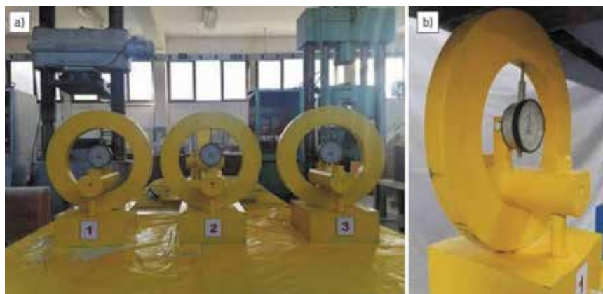
Figure 6. a) Rings with gauges for normal stress; b) Thickness of rings 1, 2 and 3 is d = 2.0 cm
