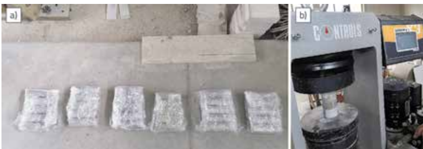
Figure 3. Examination of uniaxial strength of specimens
