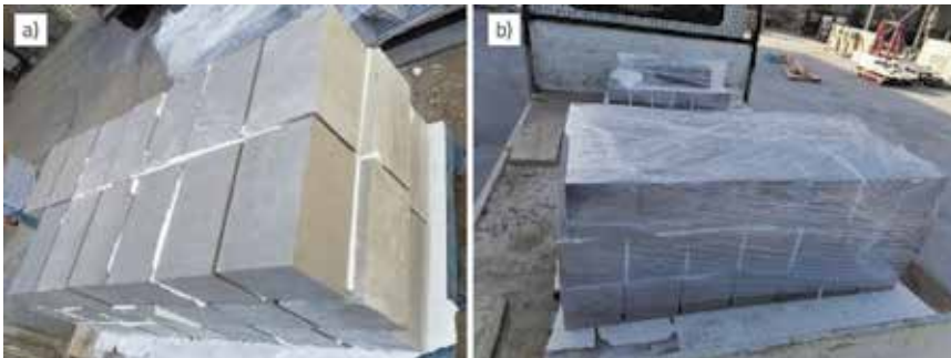
Figure 2. Specimens processed to target dimensions 30 x 15 x 15 cm
