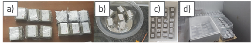
Figure 7. Stages in sample preparation shown in photos: a) prepared samples b) placing samples in a desiccator c) arranging sample in boxes d) placing samples in the freeze-thaw cabinet
