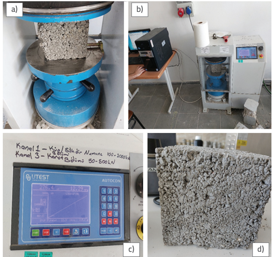
Figure 14. a) Compression test machine; b) and c) Analysis status and data obtained; d) RCC sample as a result of the test
